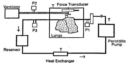
Fig. 1. Simplified diagram of the isolated lung preparation. Lungs are suspended to a force transducer fixed at the top of an humidified and temperature controlled perspex box.
