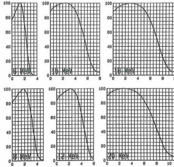
Depth dose curves for electron beams of 6, 9, 12, 15, 18 and 20 MeV, using a custom design IORT cone of 8 cm in diameter and at a source tumor distance of 116 cm. Notice the final fall off in the dose deposit of this radiation type.
